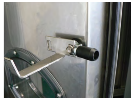
Door high pressure protection (pressure guard)
