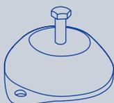
Anti-vibration kit installed under the unit to reduce transmission of vibrations
