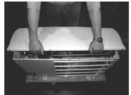
remove the roof
